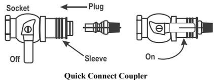
1. Insert the plug and release the sleeve.
