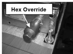
**DO NOT** remove boot. Removal of rubber boot will void manufacturer’s warranty. Rubber boot removed from end of motor only to show brake lever and spring lock.
