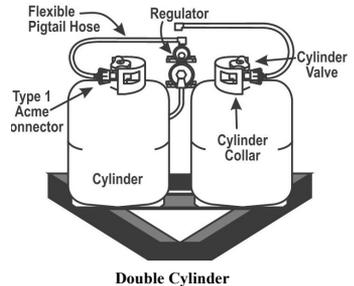
1. Secure the second cylinder to the A-frame using the bolts, nuts and washers provided.
